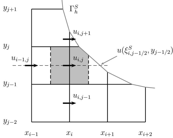
Figure 4: Five-point stencil, using the boundary condition on the obstacle  $\Gamma_h^S$ , for the first-order finite difference approximation of  $\Delta u(\boldsymbol{\kappa}_{i,j}^{y,F})$ . We recall that, in this case,  $\boldsymbol{\kappa}_{i,j}^{y,F} = (x_i, y_{j-1/2})$ .
