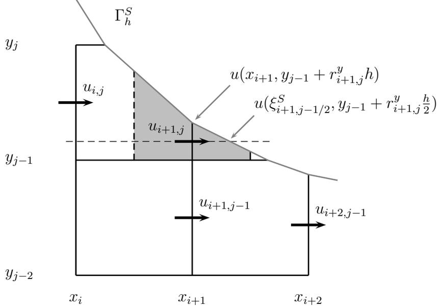
Figure 5: Six-point stencil, using the boundary condition on the obstacle  $\Gamma_h^S$ , for the first-order finite difference approximation of  $\Delta u(\kappa_{i+1,j}^{y,F})$ . We recall that, in this case,  $\kappa_{i+1,j}^{y,F} = (x_{i+1}, y_{j-1} + r_{i+1,j}^y \frac{h}{2})$ .
