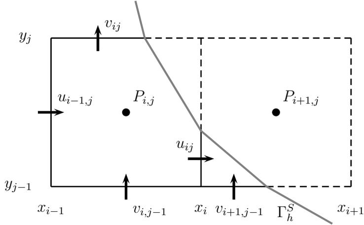
Figure 3: Location of the unknowns in the cut-cells  $K_{ij}$  (left) and  $K_{i+1,j}$  (right).
