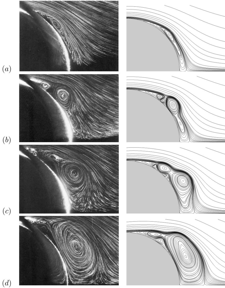
Figure 11: Flow past a circular cylinder at  $Re = 9\,500$ . Experimental results from Bouard and Coutanceau [39] (left) and streamlines obtained with the present numerical method (right). Comparison at time (a)  $t = 0.75$ , (b)  $t = 1.0$ , (c)  $t = 1.25$ , (d)  $t = 1.5$ .
