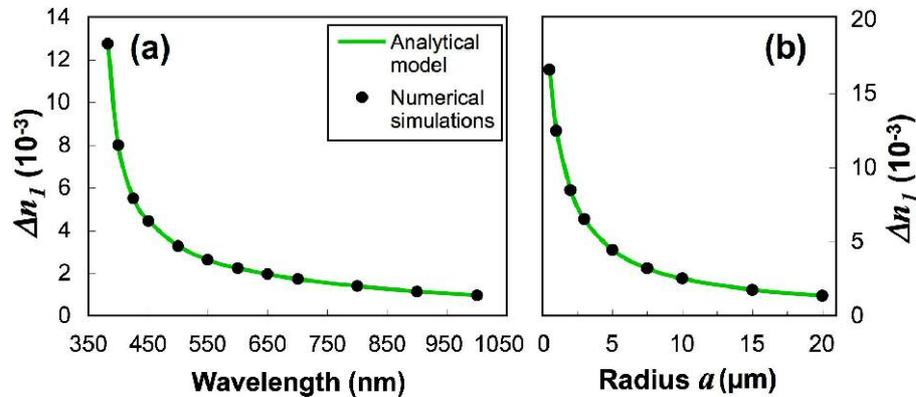
**Figure 3.** (color online) (a) Dispersion curve for the  $\text{SPP}_1$  mode (other parameter values as in Fig. 2). (b) Behavior of the effective index shift  $\Delta n_1$  versus radius  $a$  for the silver-glass convex structure of Fig. 1(b) for  $\lambda = 450 \text{ nm}$  and  $\theta = 157^\circ$ . Circles: FEM numerical results; solid curves: asymptotic analysis results.
