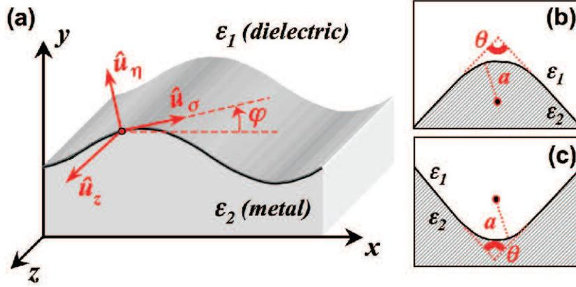
**Figure 1.** (color online) (a) Schematic of a generalized-cylinder (i.e.  $z$ -invariant) metal-dielectric interface and local curvilinear coordinate system. (b) and (c): sketch of convex and concave 'bookcover' metal-dielectric interfaces.
