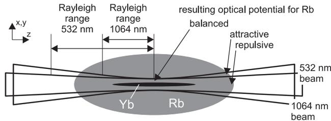
**Figure 1.** Scheme of the combined trap with the spatial configuration of the atomic clouds and the BIODT laser beams (not to scale).
