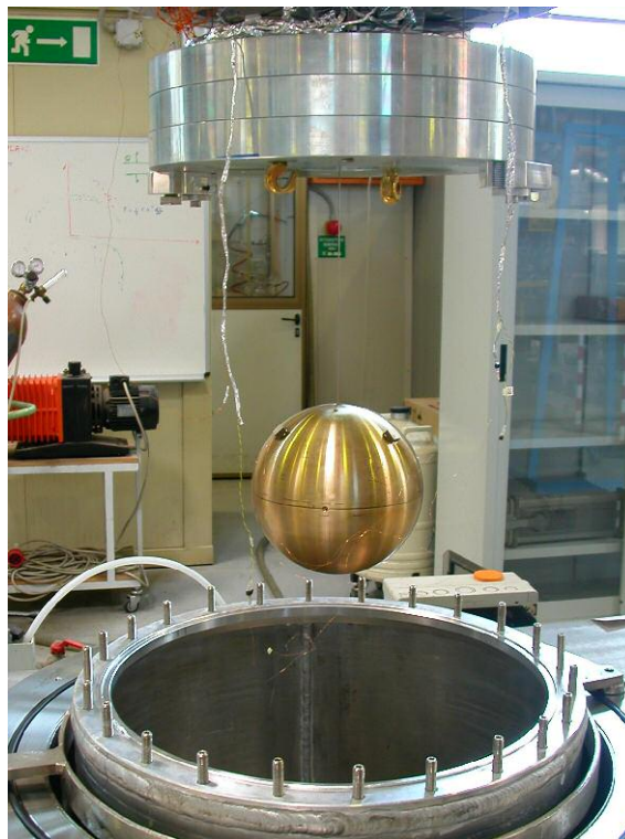
Figure 2. An image of the sphere hanging from the cold plate of the cryostat vibration isolation system. Note the suspension cable
