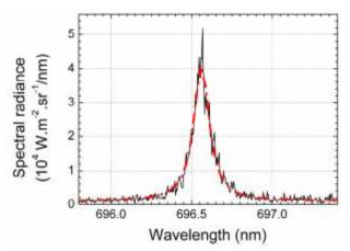
Figure 9. Lorentz line fit of the 696.5 nm argon line at t = 540 ms and lateral position Y = 0. Solid line corresponds to the experimental data, and dash line corresponds to the Lorentz profile fit.
