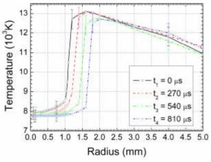
*Figure 10. Temperature profiles of the plasma at different time*  $t_i$  *of the high-current phase.*
