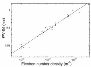
Figure 8. FWHM of the 696.5 nm argon line as function of electron number density. Circles correspond to literature values [18], and solid line corresponds to the linear fit.
