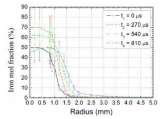
*Figure 12. Iron mol fraction at different times*  $t_i$  *of the high- current phase.*
