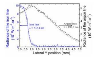
Figure 4. Radiance of the iron line at 532.4 nm and the argon line at 696.5 nm at  $t_3 = 540$  ms, as functions of the lateral Y position. Solid lines correspond to the experimental values, and dashed lines correspond to the polynomial fit values.
