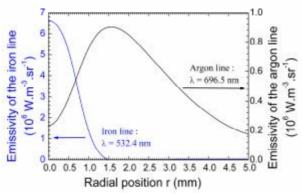
Figure 5. Emissivity of the iron line at 532.4 nm and the argon line at 696.5 nm at  $t_3 = 540$  ms, as functions of the radial position r, obtained by Abel inversion of the radiances presented in figure 4.
