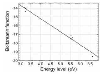
Figure 7. Example of a Boltzmann plot allowing the deduction of the plasma temperature, obtains at  $t_3 = 540$  ms, at the centre of the welding arc.
