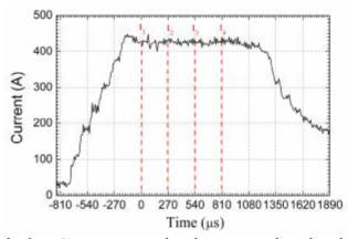
*Figure 3. Definition of the four times*  $t_1$ ,  $t_2$ ,  $t_3$  and  $t_4$  chosen to explore the whole high- current phase.
