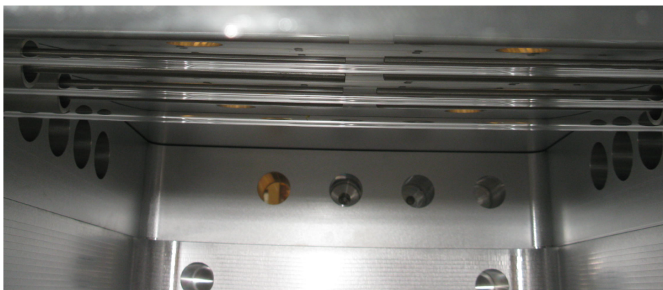
Figure 2 , Microwave plasma sources arranged parallel to one another
