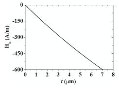
**Figure 5.** Bias field  $H_b$  created by an FeNi tube as a function of its thickness t.  $H_b$  is calculated in one point of the Fe-rich core 15  $\mu$ m from one end.  $M_s$ = 1T. The tubes are of the same length (13mm) and inner radius (19  $\mu$ m) to those in figure 2.
