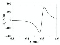
**Figure 4.** Bias field  $H_b$  created by a 7.5  $\mu$ m thick FeNi tube along the axis z of the Fe-rich core close to one of its ends (vertical dashed line).  $M_s$ = 1T. The tube is of the same length (13mm) and inner radius (19  $\mu$ m) to that one in figure 2.
