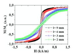
**Figure 7.** (color online) Axial hysteresis loops a 7.5  $\mu$ m thick FeNi tube as a function of its length *l*. The inner and outer radii are the same ones to those in figure 2.
