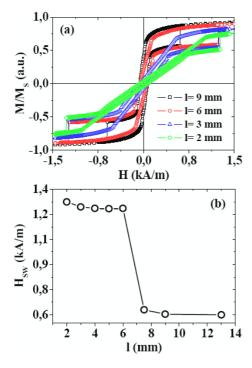
**Figure 6.** (color online) Influence of the sample length l in an FeSiBP-FeNi microwire with a 7.5  $\mu$ m thick FeNi shell. (a) Axial hysteresis loops. (b) The evolution of  $H_{sw}$ . Line is a guideline for the eye.
