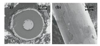
**Figure 1.** SEM images of an FeSiBP-FeNi microwire with a 2  $\mu$ m thick outer FeNi shell. (a) cross section and (b) side view showing the outer FeNi layer.
