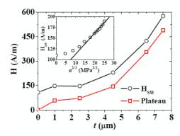
**Figure 3.** (color online)  $H_{sw}$  (black circles) and extent of the plateau (red squares) in FeSiBP-FeNi microwires as a function of the thickness t of the outer FeNi shell. Lines are guidelines for the eye. Inset shows the dependence of  $H_{sw}$  on applied tensile stress in the bare FeSiBP microwire. Line represents a linear fit.
