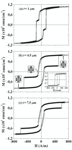
**Figure 2.** Axial hysteresis loops of FeSiBP-FeNi microwires as a function of the thickness t of the outer FeNi shell: (a)  $t=1\mu m$ , (b)  $t=4.5\mu m$ , (c)  $t=7.5\mu m$ . t=13 mm. Inset shows the hysteresis loop of the bare FeSiBP glass-coated microwire.
