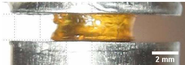
Figure 4: Photograph of binder disc, between the bars. The bar diameter, 12.7 mm, acts as a scale for measuring the specimen dimensions.
