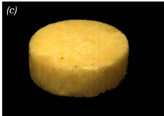
Figure 7. Photographs of PBX specimens (a) undamaged; (b) compressed to 3% strain at -70^{\circ}\text{C} ; (c) compressed to 3% strain at 22^{\circ}\text{C} ; (d) same specimen as figure (c), stained with blue dye to illustrate shear-banding. Scale shown in (a) also applies to (b) and (c).
