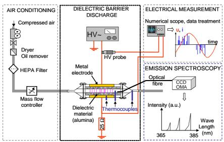
Figure 1: Experimental setup for electrical and thermal characterizations.
