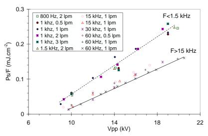
Figure 6: Mean surface energy density per period at different frequencies from 0.8 to 60 kHz, 0.5 mm gap.
