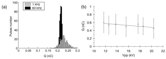
**Figure 2:** (a) Frequency distributions of charge per filament at 1 kHz (P=1 Watt, Tel=25 K) and 60 kHz (P=20 Watts, Tel=150 K) for the 0.5 mm gap length DBD at 4 lpm (b) Mean charge per filament versus applied peak-to-peak voltage, the error bars correspond to standard deviation, 1 mm gap, at 60 kHz and 1 lpm.
