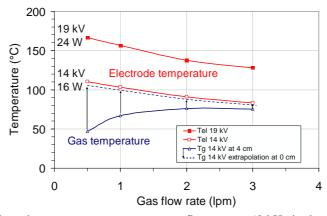
Figure 4: Electrode and gas temperatures versus gas flow rate at 60 kHz in the 0.5 mm gap DBD.
