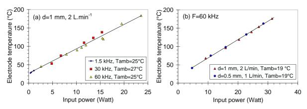
**Figure 3:** Electrode temperature versus input power (a) at different frequencies of applied voltage 1.5, 30 and 60 kHz (b) for 0.5 and 1 mm gap length at constant gas flow velocity.
