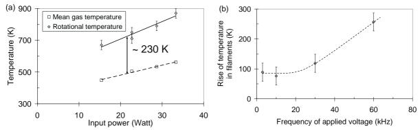
**Figure 5:** (a) Mean temperatures of gas and plasma versus input power (60 kHz) (b) Temperature rise in the filament versus frequency.
