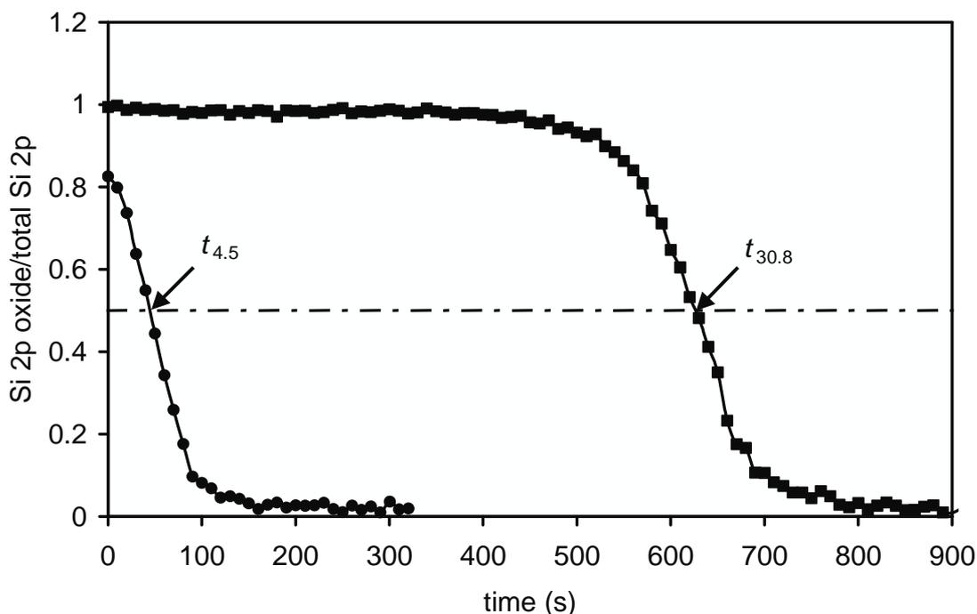
**Figure 9.** Depth profiles of the 30.8 nm and 4.5 nm oxides using the ratio of the Si 2p oxide intensity to the total Si 2p intensity, showing the times  $t_{30.8}$  and  $t_{4.5}$  determined at the 50% ordinate level.
