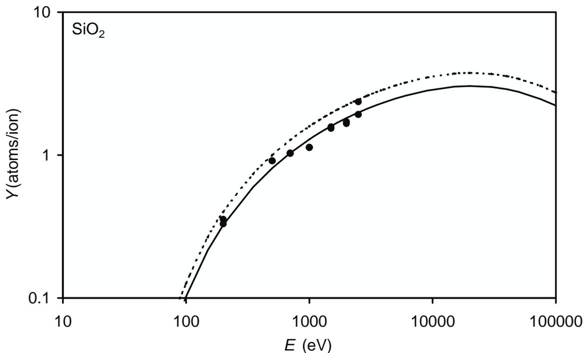
**Figure 10.** The sputtering yield  $Y(\infty)$  for  $\text{SiO}_2$  using argon ions at normal incidence. The dashed curve is the result for the semiempirical equation with interpolated parameters, and the solid curve is that result scaled by  $0.81$ .
