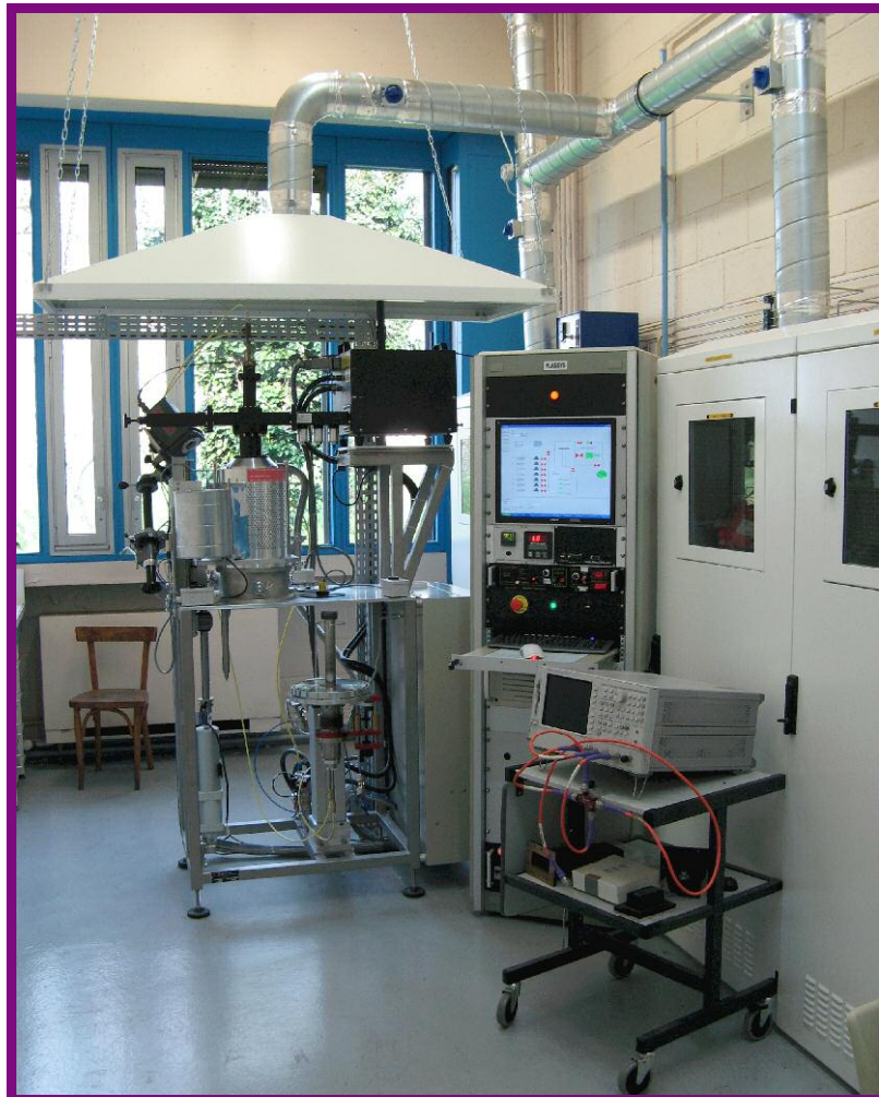
Figure 1 : experimental set up for diamond growth.
