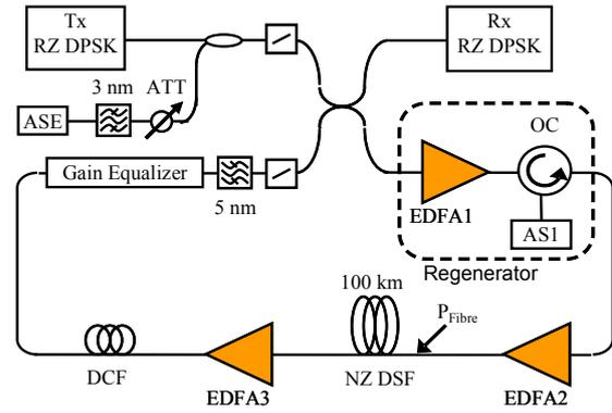
**Fig. 4:** Recirculating loop experiment of cascaded microcavity-saturable-absorber-based regenerator.
