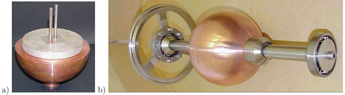
FIG. 2. a) Picture of one hemisphere of the inner sphere. Different pieces of magnets in gray are assembled in the bulk of the inner sphere. b) View from the side of the inner sphere and its rotating shaft. Note that the wheels at the top and bottom (only one is shown in the picture) of the rotating shaft are attached to the outer sphere.
