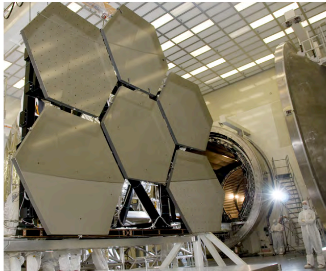
Figure 39. Six of the 18 James Webb Space Telescope mirror segments are being prepared for a cryogenic test at NASA's Marshall Space Flight Centre. Five days are needed to cool a mirror segment to -25K, permitting engineers to measure in extreme detail how the shape of each mirror changes as it cools. From http://www.jwst.nasa.gov/images_mirror30.html . Credit: NASA/MSFC/Emmett Givens.
