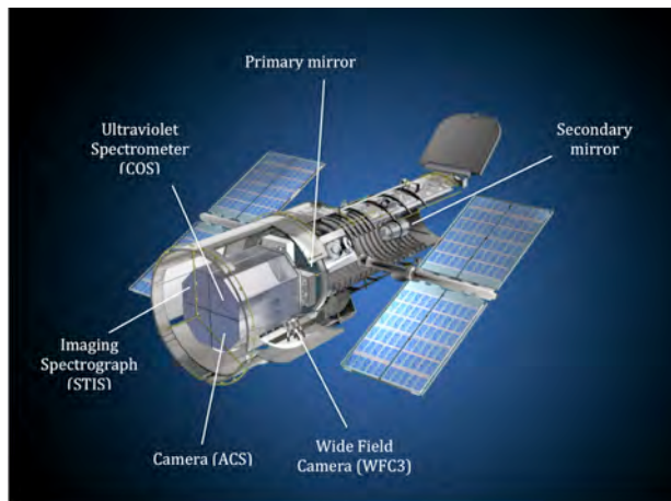
Figure 20. View of Hubble showing the instruments and the whole system. Adapted from http://www.spacetelescope.org/images/exploded_view/ . Credit: ESO.
