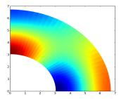
Figure 8: The magnetizing field H in physic domain with boundary conditions on perfect conductors.
