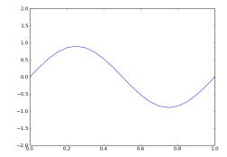
Figure 4: The magnetizing field H in 1D with perfect electric conductor boundary conditions.
