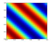
Figure 2: The first component of the electric displacement field Dx in 2D with periodic boundary conditions.
