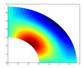
**Figure 6:** The first component of the electric displacement field Dx in physic domain with boundary conditions on perfect conductors.
