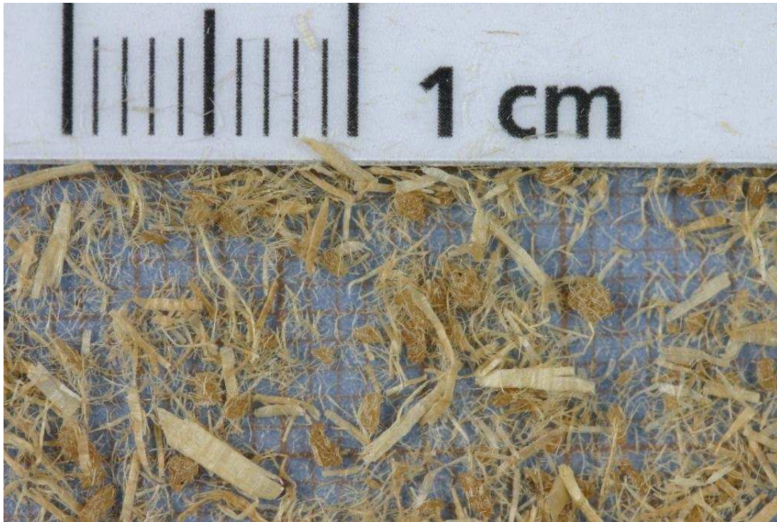
Figure 3: Extracted refiner wood fibres after compounding in a thermokinetic mixer (compound 1: 70% refiner wood fibres; 25.5% polypropylene fibres; 3% MAPP; 1.5% lubricant).
