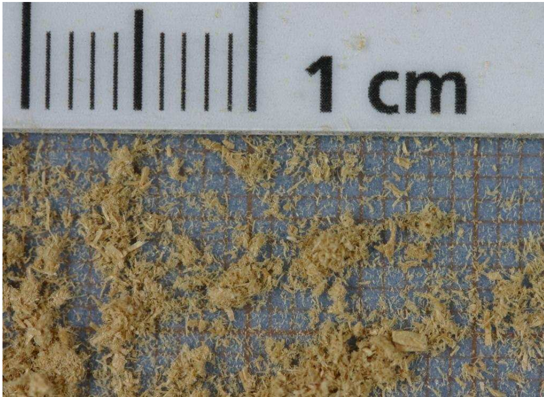
Figure 4: Extracted refiner wood fibres after extrusion (compound 1: 70 % refiner wood fibres; 25.5 % polypropylene fibres; 3 % MAPP; 1.5 % lubricant).
