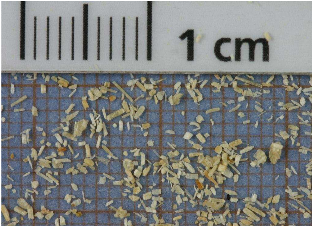
Figure 5: Extracted wood flour after compounding in a thermokinetic mixer (compound 8: 70 % wood flour; 25.5 % polypropylene fibres; 3 % MAPP; 1.5 % lubricant).
