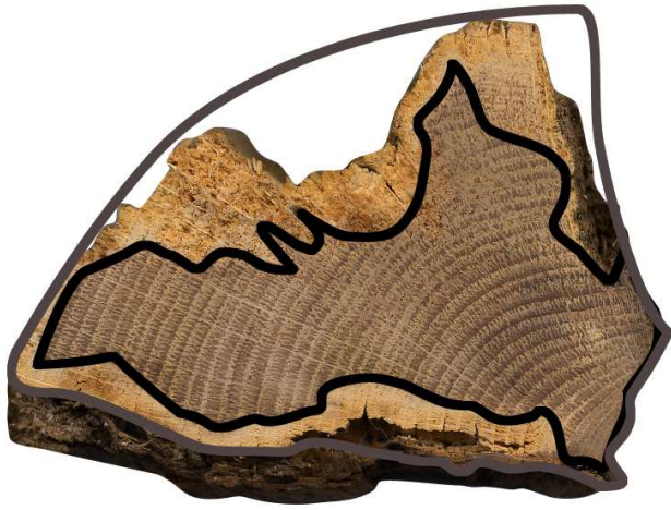
Fig. 2. Determination of remaining cross section. Grey line: Reconstructed original heartwood cross section. Black line: Remaining undecayed heartwood cross section.
