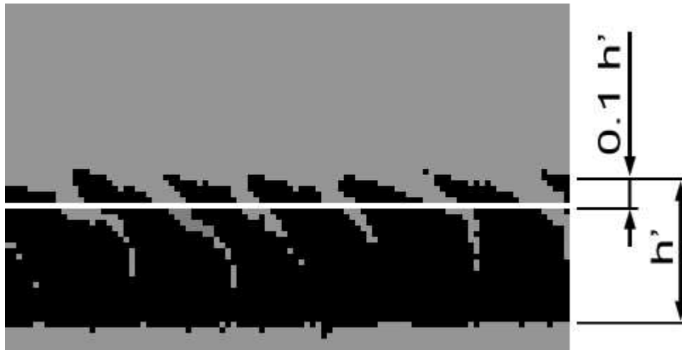
Fig. 6 Rescaled image of veneer used for Region Of Interest (ROI) extraction and coarse positions of checks determination at the specified depth of veneer – 10% of its thickness ( h' ) 176x86mm (72 x 72 DPI)
