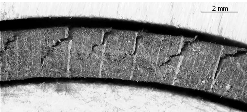
Fig.1 Lateral view of checked veneers under the microscope 202x91mm (96 x 96 DPI)
