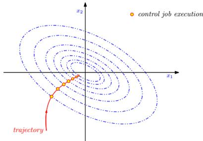
Fig. 1. Lyapunov sampling principle for a two-state system
