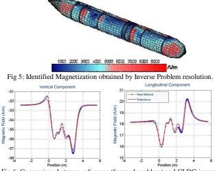
Fig.6: Comparison between reference (forward problem) and CLDG inverse problem signature prediction.
