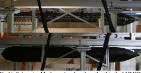
Fig 11: Submarine Mock-up placed on the railwail in the LMMCF The experimental set-up makes it possible to take measurements with an accuracy exceeding a few hundreds of
