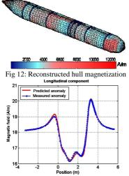
Fig 13: Results of the experimental set-up: Comparison between Measured and predicted signatures.
