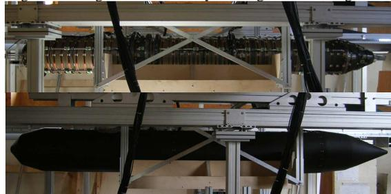
Fig 11: Submarine Mock-up placed on the railway in the LMMCF
