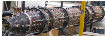
Fig 8: Coils system around the internal hull (between the 2 hulls).
