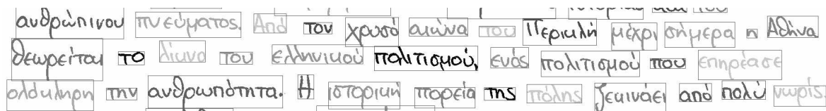
Figure 5. Words that are found by the application of the inter-word/intra-word distance threshold between connected components
