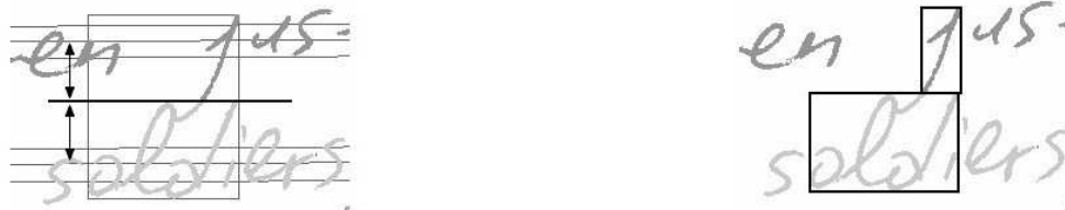
(a) One connected component that overlaps two text lines: computation of the average position of the upper and the lower middle baselines (b) Result of the segmentation: two connected components
