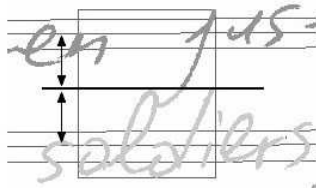
(a) One connected component that overlaps two text lines: computation of the average position of the upper and the lower middle baselines
