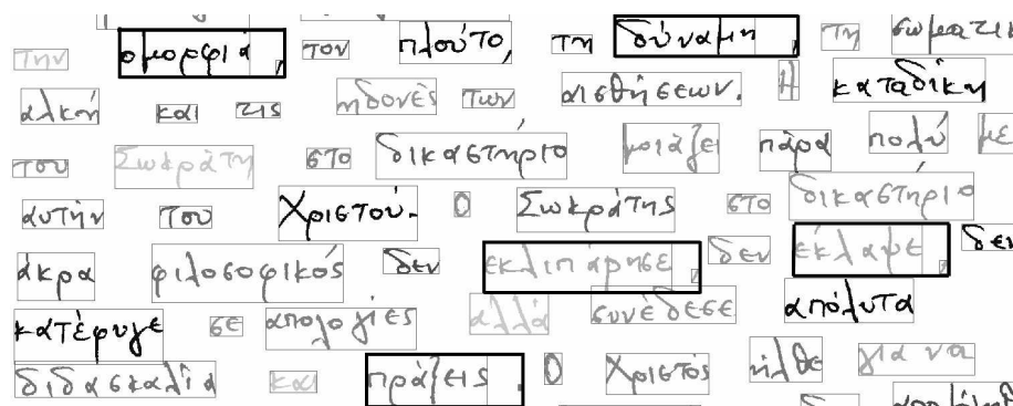
Figure 6. Introduction of structural knowledge: the punctuation is associated with the previous word (black boxes), instead of making two separate words
