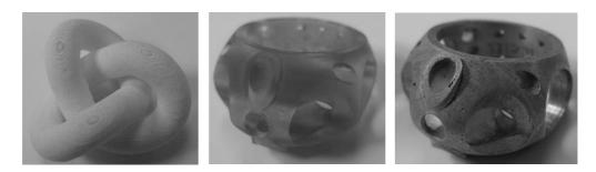
Figure 5. Artistic design supported by AF: artistic model (a), jewel model fabricated with DLP and (c) vacuum casted silver ring.
