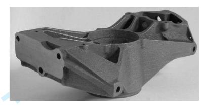
Figure 2. A race car upright fabricated with Additive Manufacturing (courtesy of Arcam).
