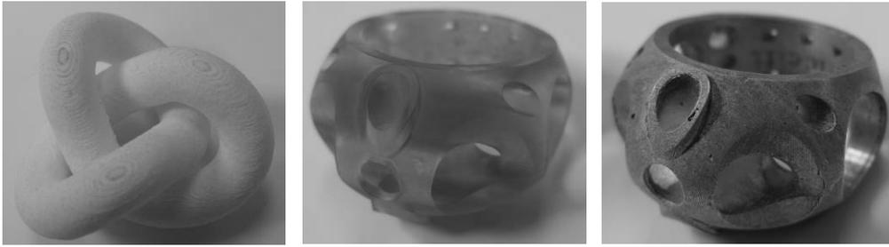
Figure 5. Artistic design supported by AF: artistic model (a), jewel model fabricated with DLP and (c) vacuum casted silver ring.
