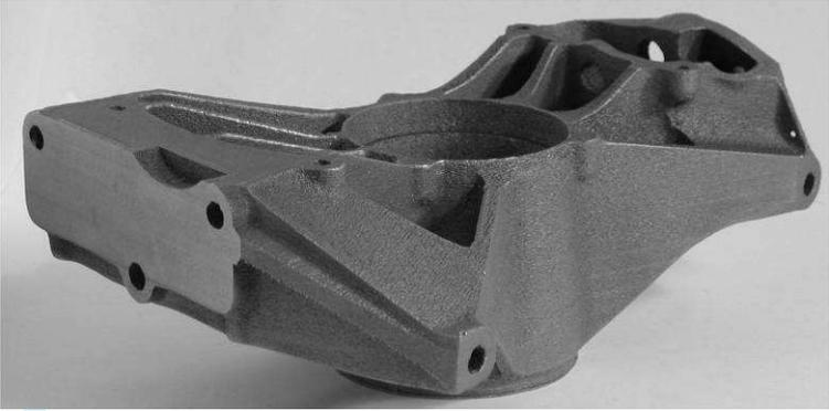
Figure 2. A race car upright fabricated with Additive Manufacturing (courtesy of Arcam).
