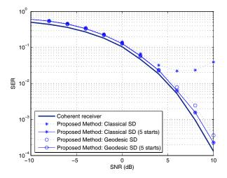
Fig. 6: Alamouti Coding: Symbol Error Rate.
