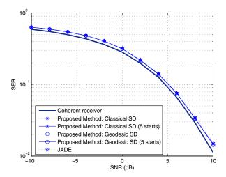
Fig. 4: Spatial Multiplexing: Symbol Error Rate.
