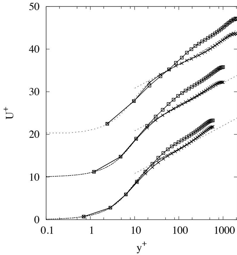
Figure 6. Streamwise mean velocity, for  $Re_+ = 590$ ,  $Re_+ = 1000$  and  $Re_+ = 2000$  from bottom to top, respectively, shifted by 10 wall units upward. Square: LES; cross: LES-SSAM; dash: DNS (only for  $Re_+ = 590$  and  $Re_+ = 1000$ ); dots: DNS from [47] for  $Re_+ = 590$  and from [48] for  $Re_+ = 1000$  and  $Re_+ = 2000$ . Long dashed line: logarithmic law of the wall.
