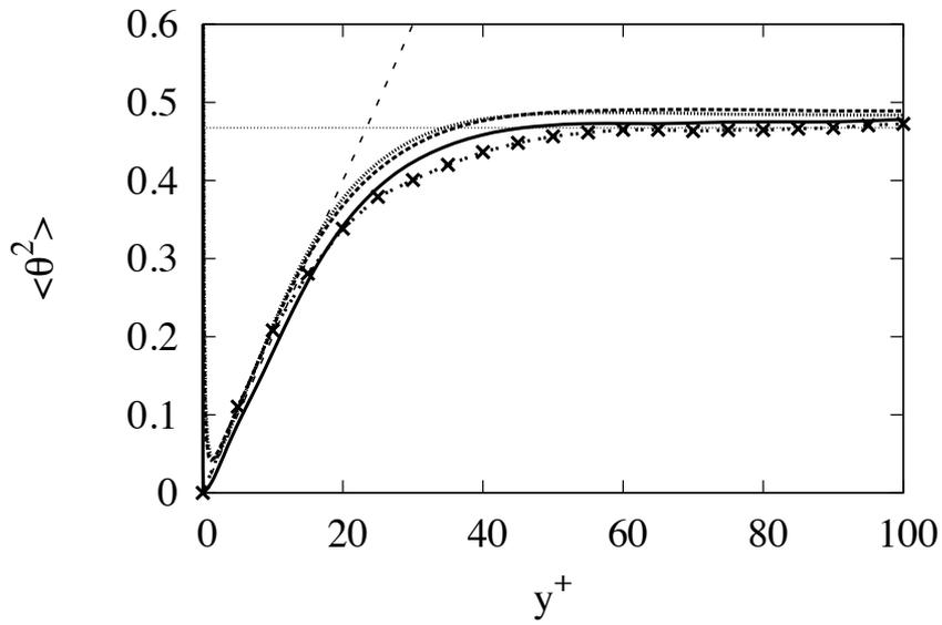
Figure 5. Evolution of the variance of  $\theta$ . Comparison between DNS for  $Re_+ = 180$  (full line)  $Re_+ = 590$  (dotted line) and  $Re_+ = 1000$  (dashed line) and the stochastic model defined by Equations 19, 20 and 22 (crosses). The straight line corresponds to the variance for an isotropic distribution.
