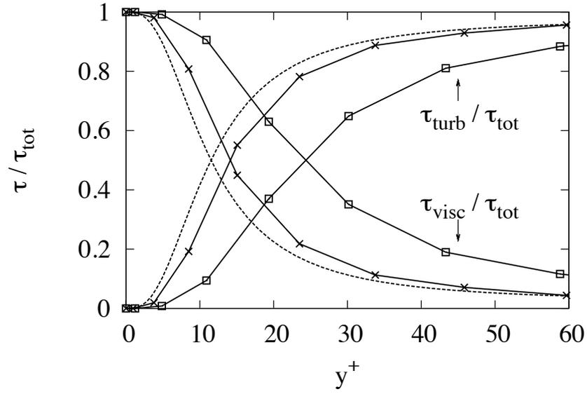
Figure 8. Ratios of turbulent  $\tau_{turb} = -\rho\langle u'v' \rangle$  and viscous  $\tau_{visc} = -\rho\nu\langle \frac{\partial u}{\partial y} \rangle$  stresses compared to the total one  $\tau_{tot} = \tau_{visc} + \tau_{turb}$ .  $Re_+ = 1000$ . Square: LES; cross: LES-SSAM; dash: DNS.
