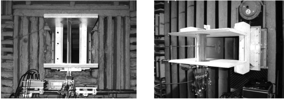
Figure 3: Experimental setups of ECL in open-jet anechoic wind tunnels with narrow (WT1) and large (WT2) rectangular nozzles, featuring the instrumented airfoils. Remote-microphone probes for wall-pressure measurements, coupling a capillary tube inside the mock-up and an external microphone, are visible below the lower side-plates.
