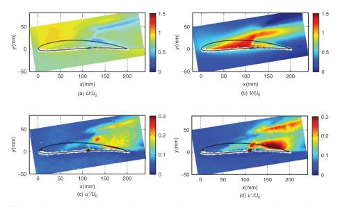
**Figure 6:** Velocity field obtained by PIV in the gap (at z = -3 mm) for the reference configuration ( $U_0 = 70$  m/s, h = 10 mm;  $\alpha = 15^\circ$ ): mean chord-wise (a); mean cross-chord (b); rms chord-wise (c); rms cross-chord (d).
