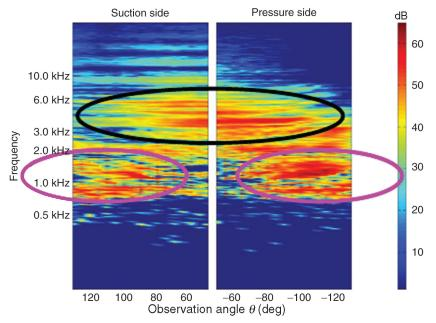
**Figure 11:** Tip clearance contribution to the far field (h = 10 mm,  $\alpha = 15^{\circ}$ ,  $U_0 = 70 \text{ m/s}$ ), against observation angle and frequency. The color scale indicates the PSD level in dB-ref 4.10<sup>-10</sup> Pa<sup>2</sup>/Hz.
