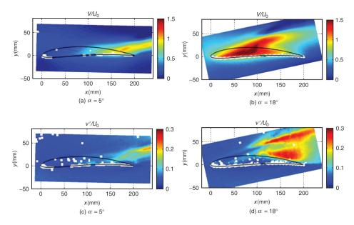
**Figure 7:** Velocity field obtained by PIV in the gap (at z = -5 mm) for 2 angles of attack  $\alpha = 5^{\circ}$  (a) (c) and  $18^{\circ}$  (b) (d) at  $U_0 = 70$  m/s and h = 10 mm: mean relative normal-to-chord velocity (a) (b) and relative rms level of normal-to-chord velocity fluctuations (c) (d). (white spots are due to light reflections on the airfoil or diffusion or to dust poarticles on the window).
