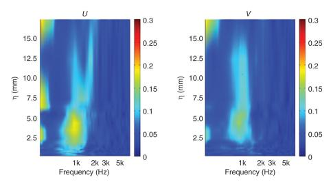
Figure 13: Coherence between the velocity measured by LDA in the plane of probe 21 (z = 1.5 mm) and the far field microphone for various LDA probe positions following line 1.  $\eta$  denotes the distance between the LDA measurement point and the wall along the measurement line.
