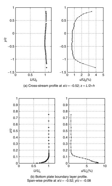
**Figure 4:** Upstream flow at 70 m/s, h = 10 mm and  $\alpha = 15^{\circ}$ .
