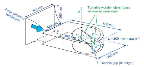
**Figure 1:** Experimental set-up. Overall picture of the pressure side showing the nozzle exit (blue), the plates with a glass window on the bottom one, the remote pressure probes (Top); sketch of the set-up with co-ordinates and rig dimensions (Bottom).
