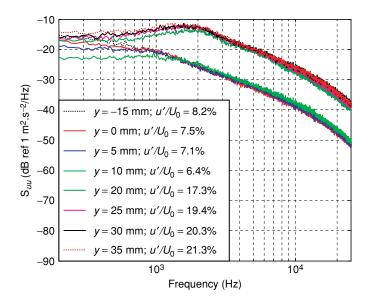
Figure 9: Spectra in the gap region at  $x/c = 0.95 \ z = -5 \ \text{mm}$  and y = -15; 0; 5; 10; 20; 25; 30; 35 \ mm:  $u'/U_0 \ (u' = 5.76; 5.24; 4.97; 4.48; 12.1; 13.6; 14.2; 14.9 \ \text{m/s respectively}) \ (U_0 = 70 \ \text{m/s}, h = 10 \ \text{mm}; \alpha = 15^\circ).$
