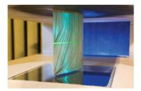
(b) Picture of the airfoil showing TE corner and (near) mid-span probes. The lines correspond to the imbedded tubes.
