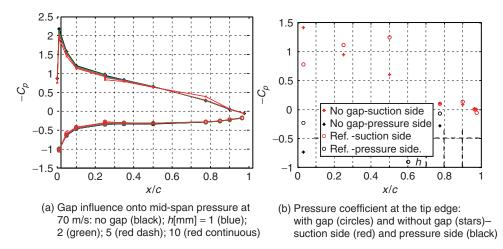
**Figure 5:** Pressure coefficient at  $U_0 = 70$  m/s, h = 10 mm;  $\alpha = 15^{\circ}$ .
