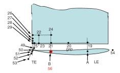
(a) Pressure probe locations in the gap and near the gap on the suction side. Pressure side probes and mid-span probes are not shown here.
