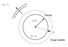
Figure 2: Noise generated by a spherically expanding flame, refer to Thomas & Williams.<sup>82</sup> A mixture of air and ethylene is used as premixed combustible gas within a soap bubble, yielding basically  $C_2H_4 + 3 O_2 \rightarrow 2 CO_2 + 2 H_2O$ . Density and speed of sound of the ambient medium as well as the mixture are  $\rho_{\infty}$  and  $c_{\infty}$  whereas those of burn gas are denoted  $\rho_b$  and  $c_b$ .
