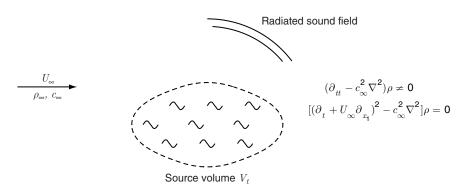
Figure 3: Noise generated by a turbulent flow surrounded by a uniform mean flow.
