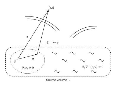
Figure 1: Sketch illustrating Lighthill's integral solution given by Eq. (14). By neglecting aerodynamic noise, the source term in the volume V basically represents the contribution of the direct combustion noise associated with the unsteady rate of heat release  $\partial_t \dot{\omega}_T$  and of the entropy noise associated with the term  $\partial_t \nabla \cdot (\rho_e u) \neq 0$ .
