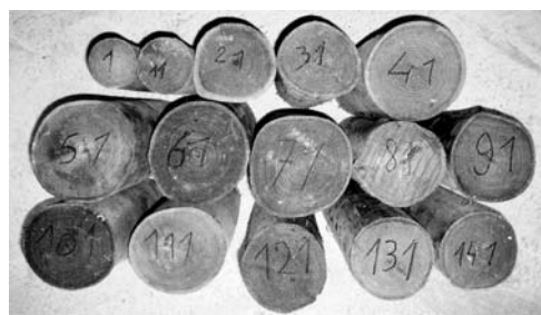
Fig. 9 Logs series treated in a 130 °C oil bath – treatment time determined using the diameter-treatment time determination chart, before natural drying to 12% moisture content
