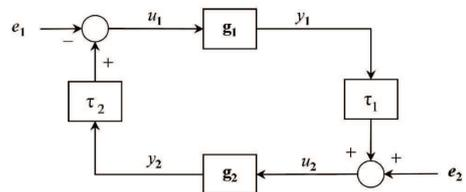
Fig. 6. Closed loop of the interconnected systems
