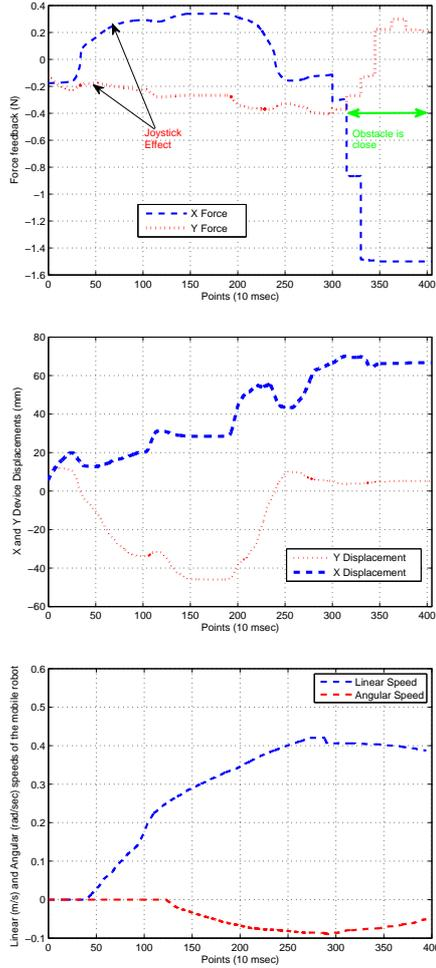
Fig. 11. Experimental Results of the Mobile Robot approaching a wall without Time Delay  $\tau_i=0$ : (a) X and Y Force feedback, (b) X and Y device displacements and Linear and angular speeds of the Mobile Robot
