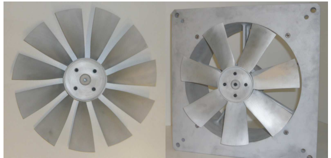
FIG. 1. Picture of the Front Rotor (left) and Rear Rotor (right)
