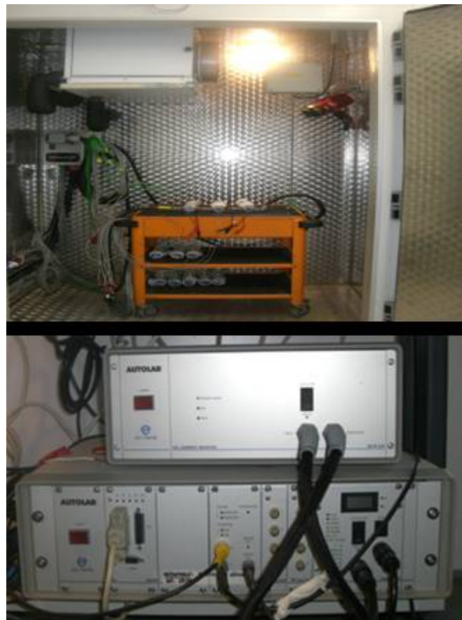
Figure 3: The climatic chamber and used measurement devices of battery impedance
