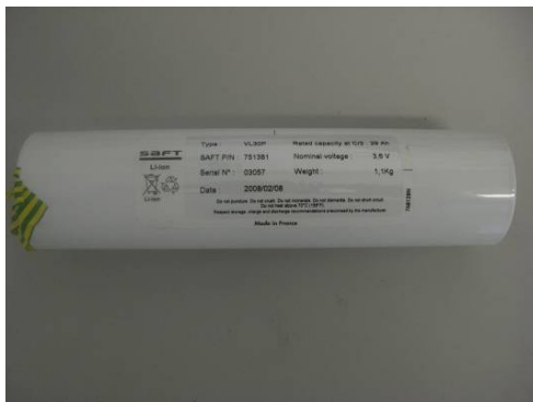
Figure 1: Lithium-ion VL30P cell from SAFT
