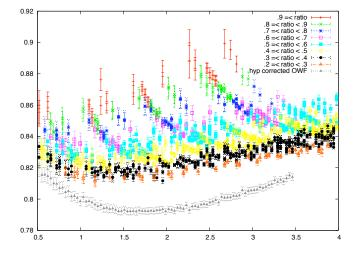
The plot on the left shows the result for  $Z_{\text{qlatt}}$  as a function of  $p^2$ stemming directly from the lattice calculation. It is very far from the smooth dependence expected in the continuum. One sees a "half-fishbone" structure which is a dramatic expression of hypercubic artefacts. Let us define
