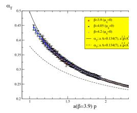
In the plot on the left we have merged the three curves of  $\alpha_T(\mu^2)$  by fitting the lattice spacing ratios to have the best matching. The compatibility of the three curves is quite impressive and the needed lattice spacing ratios agree very well with what is extracted from the interquark potential [22]. The fit has been performed both using the leading logarithm [22] (LL) and the three loop [8] ( $\mathcal{O}(\alpha^4)$ ) formula for the Wilson coefficient. The result is:
