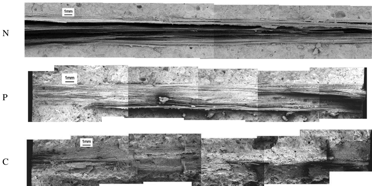
Fig 8. OC1 yarns; longitudinal sections corresponding to N, P and C impregnation.
