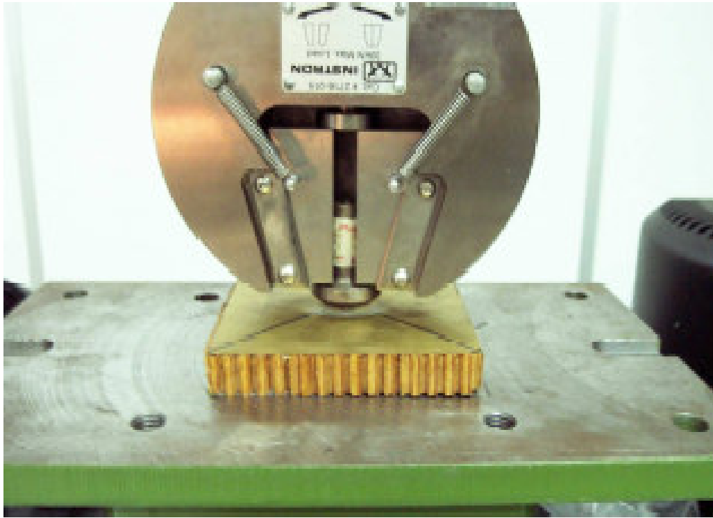
Figure 2 : Static indentation of the CAI specimens.
