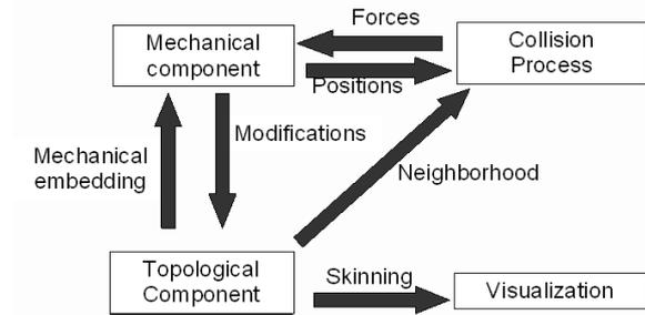
**Figure 4:** Architecture of the topologically-based mechanical model.
