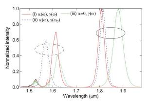
Figure 2. Output spectra (linear scale) simulated (i) with full  $\alpha(\omega)$  and full  $\gamma(\omega)$  (solid curves), (ii) full  $\alpha(\omega)$  but constant  $\gamma(\omega_0)$  (dashed curves), (iii)  $\alpha=0$  but full  $\gamma(\omega)$  (dotted curves). The pump wavelengths are 1.55 µm (solid circle) and 1.29 µm (dashed circle) (propagation distance of 50 cm).
