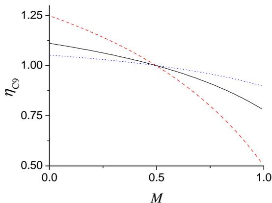
**Figure 7.** Computed  $M$ -dependence of the PE  $\eta_{C9}$  in the limit of low-intensity OP on the  $C_9$  line. Red (dashed) line:  $\eta_{C9}^D$ , high pressure limit; black (solid) line: 1.33 mbar, intermediate collisional regime; blue (dotted) line:  $\eta_{C9}^K$ , low pressure limit.
