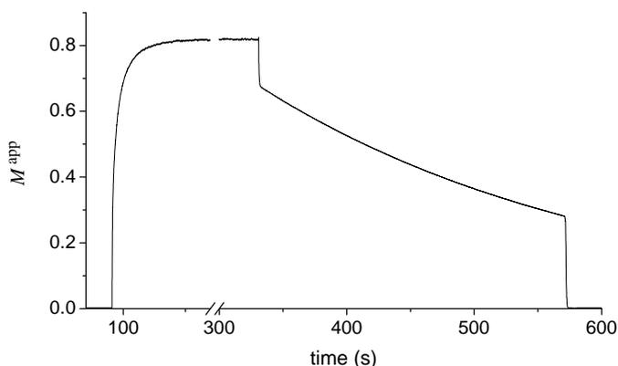
**Figure 12.** Time evolution of the apparent polarisation  $M^{\text{app}}$  in the 1.19 mbar cell, monitored using a  $C_8$ -tuned probe. OP is applied from  $t=91$  s to  $t=330$  s ( $C_8$  line,  $W_{\text{las}}=1.55$  W). At  $t=570$  s, the remaining polarisation is suddenly destroyed by enhanced nuclear relaxation (obtained by placing a small magnet close to the cell).
