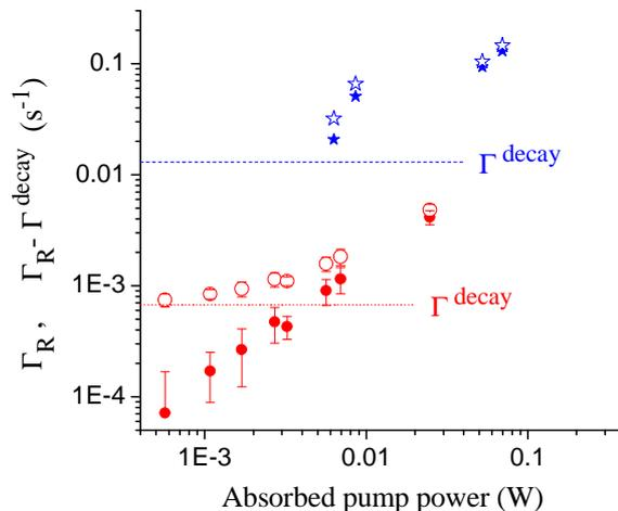
**Figure 18.** Total polarisation loss rates  $\Gamma_R$  (open symbols) for various absorbed OP powers in a 32 mbar cell, reproduced from Fig. 6.21 of [31]. The horizontal lines correspond to the measured  $\Gamma^{\text{decay}}$  values. The filled symbols are the differences  $\Gamma_R - \Gamma^{\text{decay}}$  plotted in the original figure. Blue stars and dashed line:  $B=3$  mT,  $C_9$  pump; red circles and dotted line:  $B=1.5$  T,  $f_2^-$  pump.
