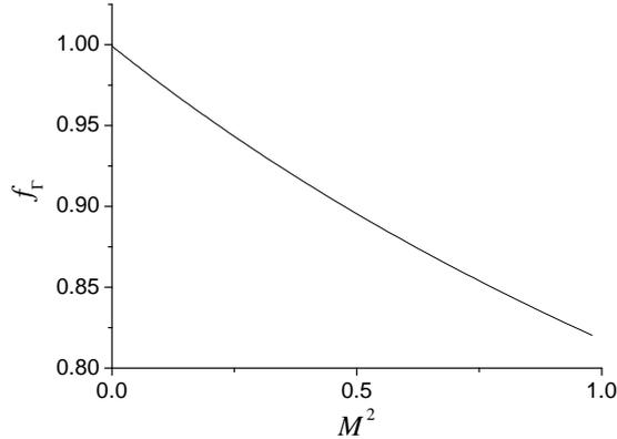
**Figure 9.** Computed decay rate factor  $f_\Gamma$  in Eq. 20 characterising the deviation of ME-induced decay of  $M$  from the small  $M$  regime of Eq. 19. The empirical fit  $f_\Gamma=0.999-0.2340M^2+0.0539M^4$  is accurate to better than  $4\times 10^{-4}$ .
