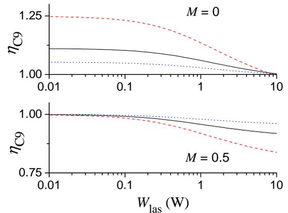
**Figure 8.** Computed power dependence of the PE of the  $C_9$  line at  $M=0$  (upper graph) and  $M=0.5$  (lower graph) for the same three collisional regimes as in Fig. 7.  $\eta_{C9}$  is here the spatial average of the PE in the cell, computed for the same pump beam parameters as in Fig. 5.
