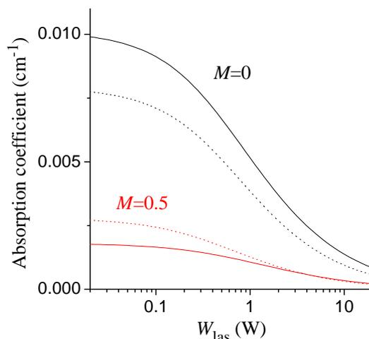
**Figure 6.** Overall pump absorption coefficients at  $M=0$  (upper black curves) and  $M=0.5$  (lower red curves) for  $C_8$  (dotted lines) and  $C_9$  (solid lines) OP, computed as a function of incident power  $W_{\text{las}}$  (same conditions as in Fig. 5).
