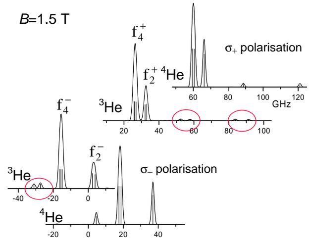
**Figure 4.** 1083 nm absorption spectra of  $^3\text{He}$  and  $^4\text{He}$  at 1.5 T for circularly polarised light. Optical transition frequencies are referenced to that of the  $C_1$  line in zero field [24]. Pump and probe lines relevant for high field MEOP are described in text.
