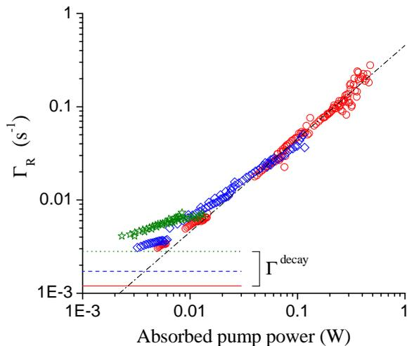
**Figure 17.** Examples of experimental total polarisation loss rates  $\Gamma_R$  obtained from polarisation build-ups (using Eq. 25) are plotted versus the absorbed OP power ( $C_8$  pumping). The horizontal lines correspond to the measured  $\Gamma^{\text{decay}}$  values. Green stars and dotted line: 0.63 mbar; blue diamonds and dashed line: 1.19 mbar; red circles and solid line: 2.45 mbar. The dash-dotted line ( $y=x/2.2$ ) is a guide for the eye.
