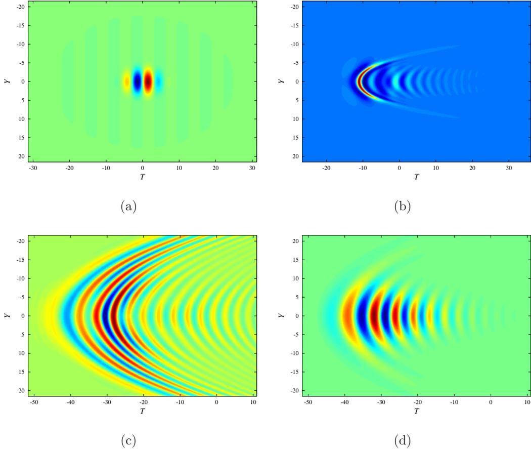
FIG. 1: (Color online) Nonlinear diffraction of a FCP. a) Initial data ( $Z = 0$ ). b) An intermediary stage, with a typical crescent shape ( $Z = 0.9594$ ). c) Nonlinear diffraction at  $Z = 3.984$ . d) Linear diffraction at the same propagation distance for comparison. Input data is expression (15) with  $p = 4.0825$ ,  $q = 2.8868$ ,  $\omega = 1$ ,  $A = 4.8990$  (a, b, c), and  $A = 10^{-7}$  (d).
