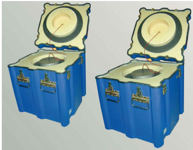
figure 1 Quasi-adiabatic calorimeters used for concrete specimens (QAB).
