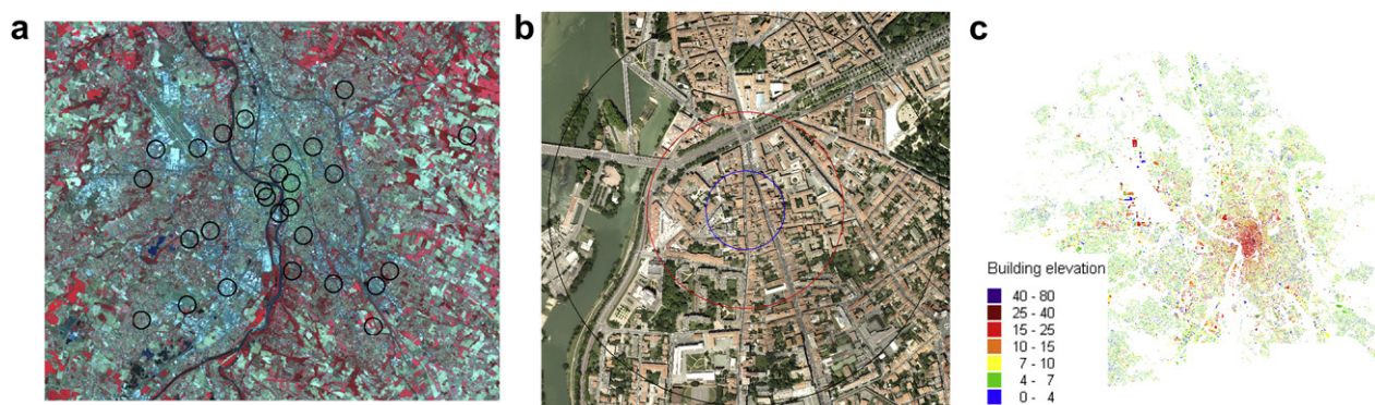
Fig. 3. Description of GIS and remotely sensed data used to compute landscape descriptors. (a) Multispectral Spot 5 imagery – Supermode 2.5 m – acquired 04/08/11 at 10:43:50 UT; (b) Aerial photographs (0.5 m) on the reference sample (MIC) with areas of 500 m (black), 250 m (red) and 100 m (blue) radius circles; (c) Building elevation data (in meters) (For interpretation of the references to color in this figure legend, the reader is referred to the web version of this article.).
