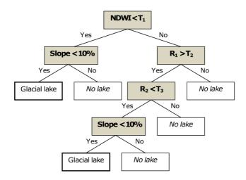
Figure 4: Algorithm to automatically classify glacial lakes on LANDSAT images, using a decision tree.  $T_i$  represents a threshold, whose value is determined empirically on each scene by visual inspection.
