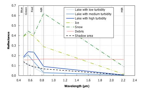
Figure 3: Spectral signatures of several recurrent terrain features of the HKH, based on a LANDSAT-ETM image from November 2001 (Bhutan). Wavelength of LANDSAT-TM and ETM channels are indicated with gray bars.
