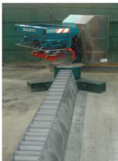
Fig. 1: CEMIB device photograph, with a real spreader coupled for testing.
