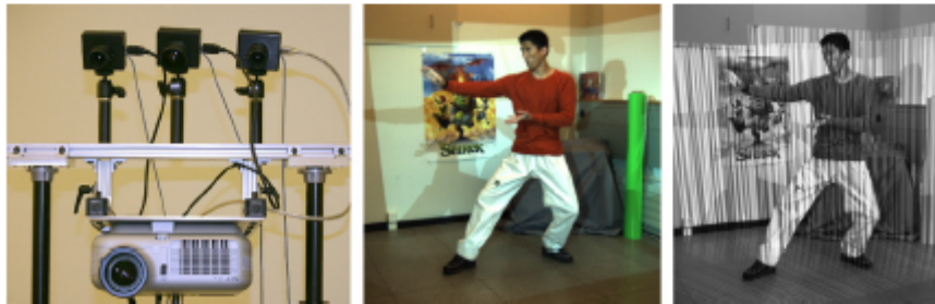
Figure 2.15: Overview of the Waschbüch 3D video framework (top) and illustration of a brick (bottom left), simultaneously acquiring textures (middle) and structured light patterns (right), from [3]
