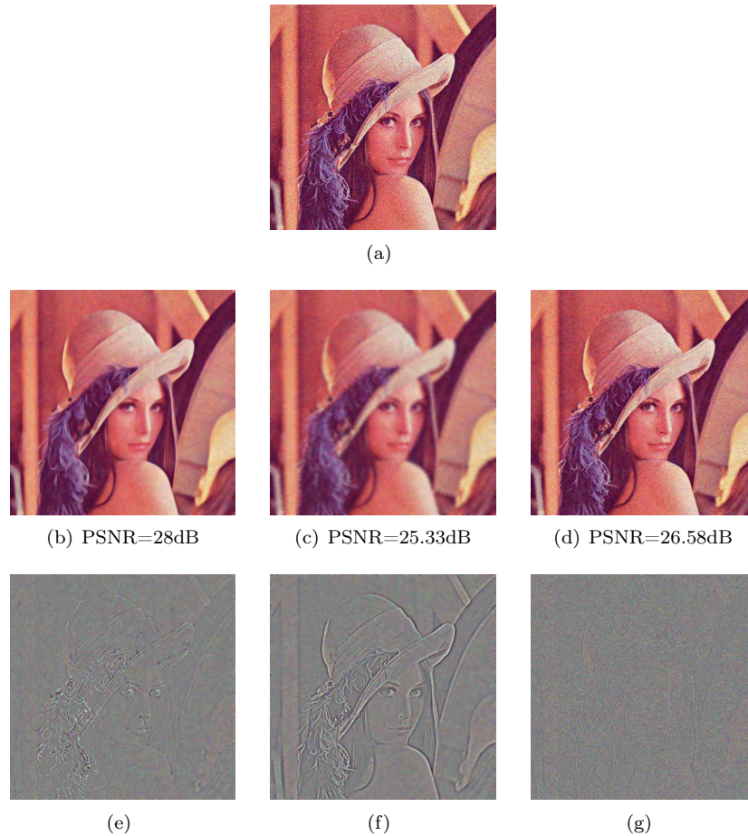
Figure 3: (a) Original picture corrupted with a gaussian Noise; (b), (c) and (d) are the filtered picture with the anisotropic diffusion proposed by Tschumperlé [71]: \mathbf{T} = c_1 \mathbf{u}\mathbf{u}^T + c_2 \mathbf{v}\mathbf{v}^T ; (b) c_1 = 0 and c_2 = 1 , Mean curvature flow; (c) c_1 = 1 and c_2 = 0 ; (d) c_i are function of the eigen values, respectively. The last row shows the residual picture (difference between original picture uncorrupted by noise and the filtered picture).
