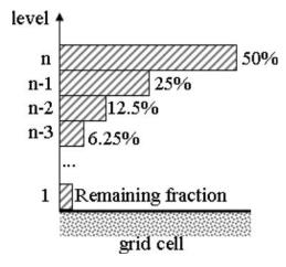
**Figure 6.** Vertical distribution of the Russian fire emissions used in simulations d, e and f. n corresponds to the maximum level at which emissions are injected. 50% of the emissions are injected at that level, half of the remaining fraction (i.e., 25%) is injected in the level below, and so on, until the first level (D. Lavoué, personal communication, 2006). Three maximum injection height are tested (3, 4.5 and 6.5 km).
