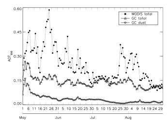
**Figure 3.** Daily total AOT $_{550}$  retrieved from MODIS observations (black dots), simulated with the GEOS-Chem model (open triangles), and simulated dust AOT $_{550}$  (open diamonds). For consistency with the rest of the study, we averaged the data over the region  $40-70^{\circ}$ N and  $140-220^{\circ}$ E (see the white box in Figure 2 and discussion in section 4).
