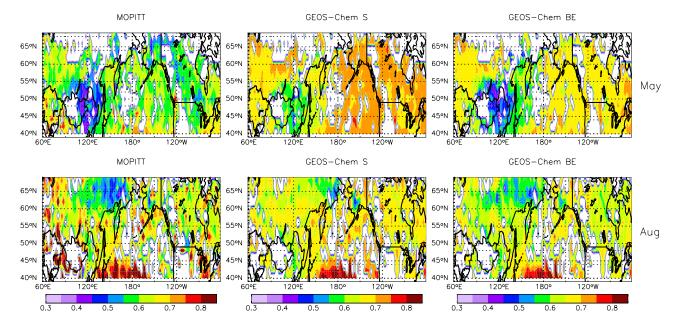
**Figure 10.** Mean monthly ratios of MOPITT CO mixing ratios between 250 and 700 hPa for May and August 2003. No data are shown for cloudy pixels or for background conditions where the CO mixing ratios is less than 100 ppbv at both levels (in order to sample only recent plumes).
